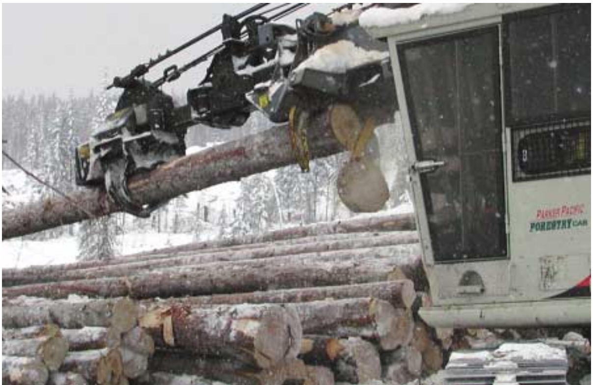
Figure 2 Processor at a Babine Forest Products roadside harvest operation long butting for excessive flare.
